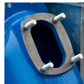
Inspection cover on volute
